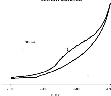
Fig. 4: Cyclic voltammogram in 2.3 mM temazepam's hydroalcoholic solution in 1.0 M HNO<sub>3</sub>; at poly-*p*-aminophenol-*p*-phenylenediamine electrodeposited on carbon. Electrode coatings obtained after 30 scans between -0.1 and -1.2 V in 100 mM each of *p*-aminophenol and *p*-phenylenediamine, Scan rate 100 mV/s, Potential vs. Saturated Calomel electrode. Curve 2 only is shown. Background curve 1 is not shown.
