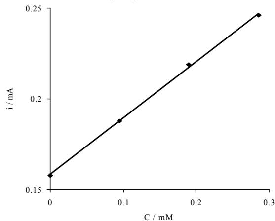
Fig. 10: Linear sweep voltammetric current at poly-*p*-aminophenol coated carbon electrodes at -0.65 V vs. concentration of temazepam in 1.0 M HClO<sub>4</sub> + 20 mM HNO<sub>3</sub>.  $y = 0.0295x + 0.1584$ ,  $R^2 = 0.9992$ . Coating conditions as per figure 8.
