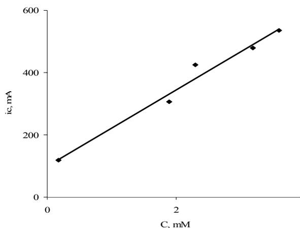
Fig. 6: Variation of cathodic current with concentration of temazepam's hydroalcoholic solution in 1.0 M HNO<sub>3</sub>; at poly-*p*-aminophenol-*p*-phenylenediamine electrodeposited on carbon in 1.0 M HNO<sub>3</sub>. Electrode coatings obtained after 30 scans between -0.1 and -1.2 V in 100 mM each of *p*-aminophenol and *p*-phenylenediamine, Potential vs. Saturated Calomel electrode,  $y = 122x + 100.54$ ,  $R^2 = 0.9748$
