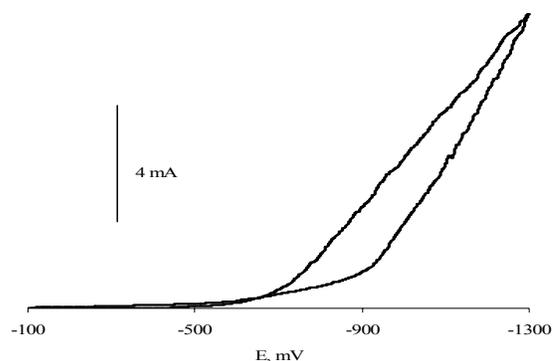
Fig. 3: Cyclic voltammogram at bare carbon in 0.17 mM hydroalcoholic solution of temazepam in 1.0 M HNO<sub>3</sub>. Electrode coatings obtained after 30 scans between -0.1 and -1.2 V in 100 mM each of *p*-aminophenol and *p*-phenylenediamine, Scan rate 100 mV/s, Potential vs. Saturated Calomel electrode.
