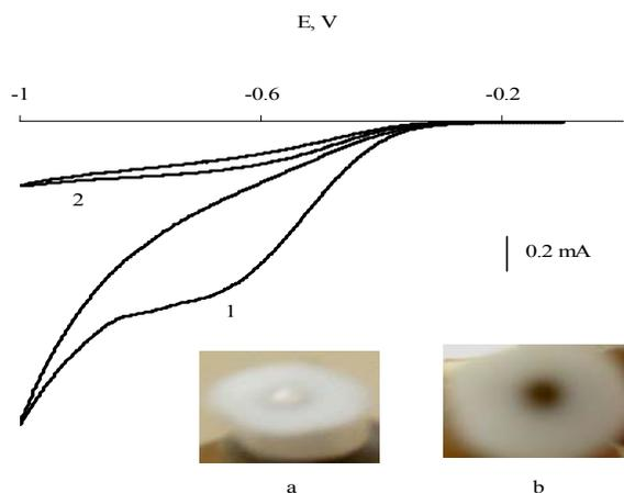
Fig. 7: Cyclic voltammograms at titanium cathodes from polymerization mixture, 100mM each of *p*-aminophenol and *p*-phenylenediamine in 1.0 M HNO<sub>3</sub>, 1<sup>st</sup> cycle (1) 50<sup>th</sup> cycle (2); Electrode surface is shown as inset before (a) and after (b) electrocopolymerization, Scan rate, 100 mV. Potential vs. Ag / AgCl, Cl<sup>-1</sup>.
