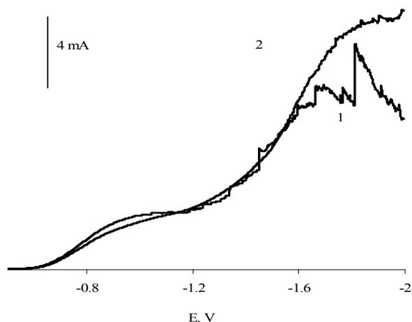
Fig. 8: Linear sweep voltammetric response in 1.0 M HNO<sub>3</sub> at (1) bare carbon, and at films of poly-*p*-aminophenol and *p*-phenylenediamine (2). Films electrodeposited on carbon by fifty successive cyclic voltammetric scans between -0.1 to -1.0 V, Scan rate, 100 mV/s, Potential vs. Saturated Calomel electrode.
