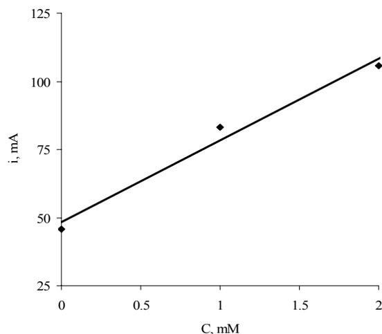
Fig. 12: Differential pulse voltammetric currents vs. concentration of temazepam in 1.0 M HClO<sub>4</sub> + 20 mM HNO<sub>3</sub> at *p*-aminophenol modified carbon electrodes, Potential vs. Ag/AgCl, Cl<sup>-</sup> at scan rate 5 mV/s, pulse height 70 mV, step time 0.4 s, pulse width 50 ms. Coating conditions as per figure 8.  $y = 30.07x + 48.207$ ,  $R^2 = 0.9805$
