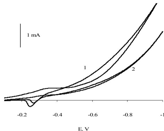
Fig. 1: Cyclic voltammetric curves at carbon cathodes from polymerization mixture, 100mM each of p-aminophenol and p-phenylenediamine in 1.0 M  $\text{HNO}_3$ , 1<sup>st</sup> cycle (1) 80<sup>th</sup> cycle (2); Scan rate, 100 mV. Potential vs. Ag / AgCl,  $\text{Cl}^-$ .
