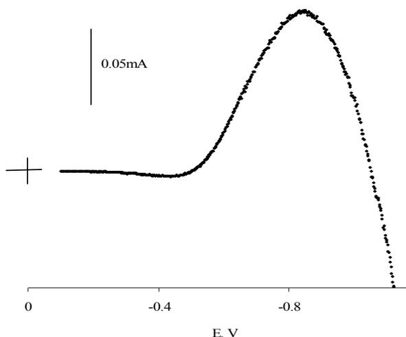
Fig. 11: Background subtracted differential pulse voltammograms at poly-*p*-aminophenol coated carbon electrodes for the reduction of 0.19 mM temazepam in 1.0 M HClO<sub>4</sub> + 20 mM HNO<sub>3</sub>, Potential vs. Ag/AgCl, Cl<sup>-</sup> at scan rate 5 mV/s, pulse height 70 mV, step time 0.4 s, pulse width 50 ms. Coating conditions as per figure 8.
