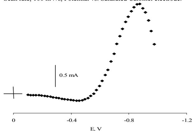
Fig. 9: Background subtracted linear scan current potential curve at poly-*p*-aminophenol coated carbon electrodes for the reduction of 0.19 mM temazepam in 1.0 M HClO<sub>4</sub> + 20 mM HNO<sub>3</sub>. Electrode coatings were obtained after 30 scans between -0.1 and -1.2 V in 6.5 mM *p*-aminophenol in 1.0 M HNO<sub>3</sub> at scan rate 100 mV/s. Potential vs. Ag / AgCl, Cl<sup>-1</sup>.
