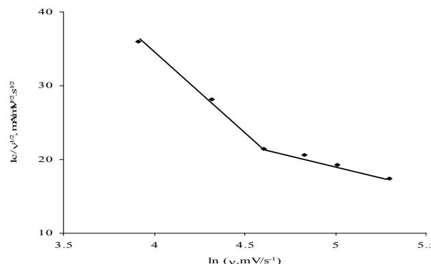
Fig. 5: Current function versus natural log of sweep rate plot for the cathodic linear sweep scan of 2.3 mM temazepam's hydroalcoholic solution in 1.0 M nitric acid. Electrode coatings obtained after 30 scans between -0.1 and -1.2 V in 100 mM each of *p*-aminophenol and *p*-phenylenediamine, scan rate 100 mV/s, potential vs. Saturated calomel electrode. Line is drawn to aid the vision, and is not a fit.
